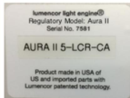
**Figure 1.** Model and serial number identification label on the AURA light engine rear panel.
