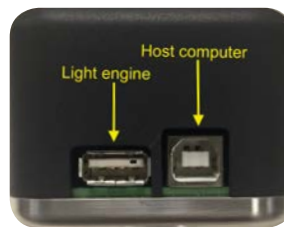
FIGURE D: USB connectors on rear of the light engine control pod
