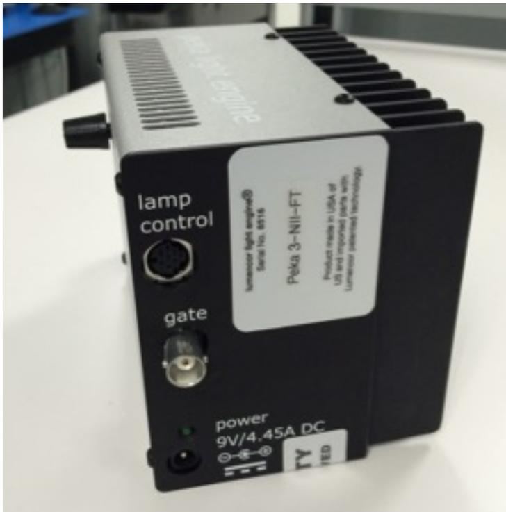
**Figure 3.** Rear panel of PEKA light engine configured for remote control from Nikon microscope base.
