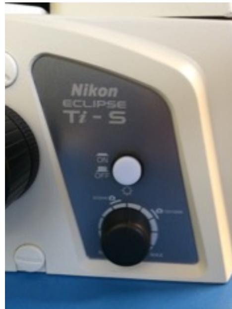
**Figure 4.** On/off and intensity controls on Nikon microscope base
